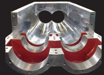
NEW CHROME PLATED BARREL SECTION OF TWIN SCREW SHEETER
