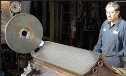
INTERNAL MIXER DOOR TOP REBUILDING
