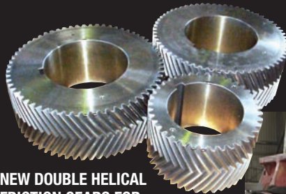
REBUILT GEAR SET FOR AN EXTRUDER APPLICATION
