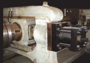
MILL CONVERSION TO HYDRAULIC ROLL NIP POSITIONING WITH SAFETY FEATURES
