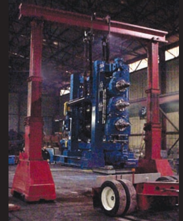
IN-HOUSE CRANE CAPABILITIES LOADING OF NEW THREE ROLL CALENDER
