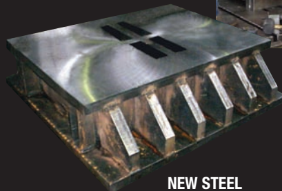
MACHINING OF NEW MILL BEARING HOUSING
