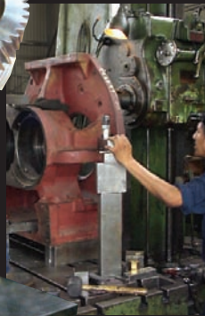
INTERNAL MIXER END FRAME REPAIR
