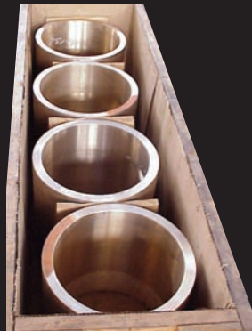
NEW REPLACEMENT BRONZE MILL BEARING LINERS
