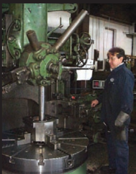
MACHINING OF NEW MILL BEARING HOUSING
