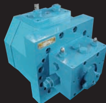
REBUILT ROTARY ACTUATOR FOR MIXER
